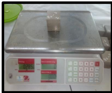
Figura 89 Pesado Mortero Experimental E3_{(1)} - 3 = 285.00 \text{ gr}
