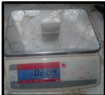
Figura 215 Pesado Mortero Experimental E3_{(1)} - 28 = 284.00 \text{ gr}
