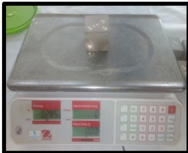
Figura 57 Pesado Mortero Experimental E1_{(1)} - 3 = 285.00 \text{ gr}
