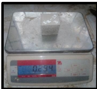
Figura 199 Pesado Mortero Experimental E2_{(1)} - 28 = 2840.00 \text{ gr}
