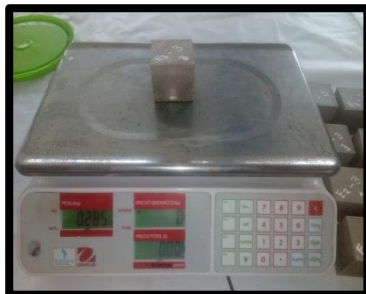
Figura 91 Pesado Mortero Experimental E3_{(1)} - 3 = 285.00 \text{ gr}
