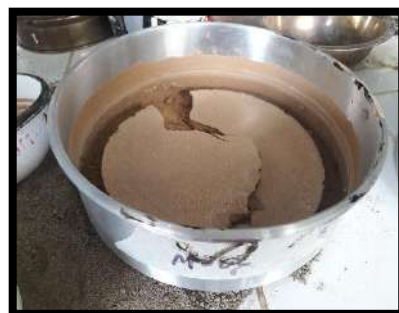
Foto 9, 10, 11, 12, 13, 14, 15, 16. Secado de la Arcilla a 110°C.
