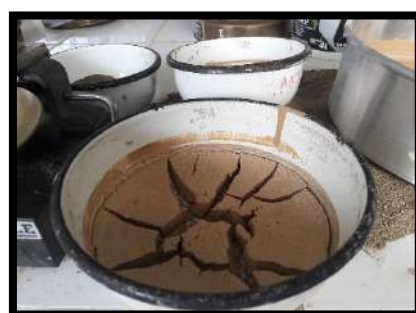
Foto 9, 10, 11, 12, 13, 14, 15, 16. Secado de la Arcilla a 110°C.
